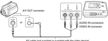
AV cable (not supplied or supplied with the video device)
